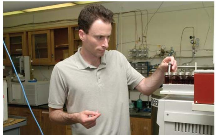
Gavin Sacks with analytical equipment (GC-MS or Gas Chromatograph-Mass Spectrometer) needed to measure low concentrations MPs.
