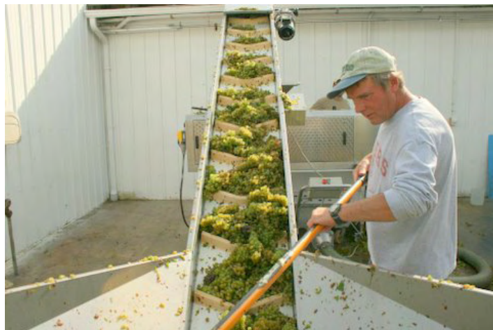
Finger Lakes: Conveying fruit to the crusher/destemmer at Hosmer Winery, Cayuga Lake.
