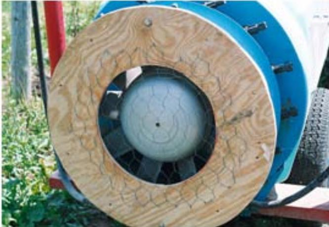
**Figure 1:** Cornell “doughnut” used to restrict airflow from airblast sprayer fan.
