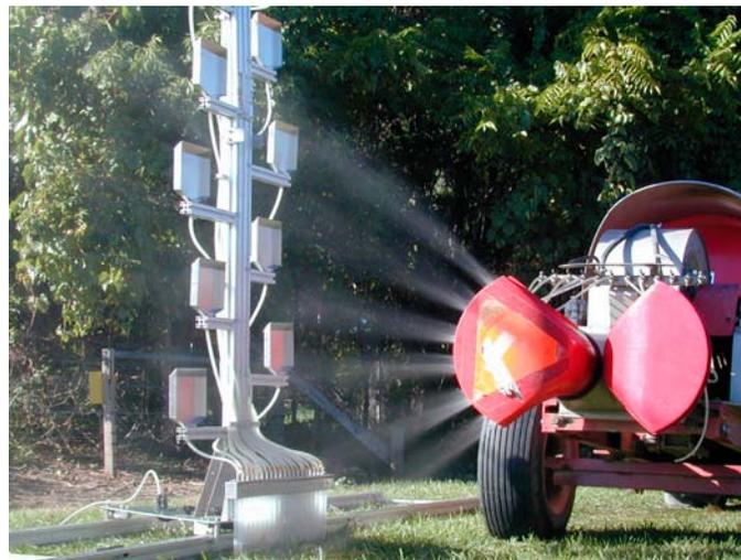
*Figure 4: Research patternator with 'air shear' Kinkelder sprayer.
