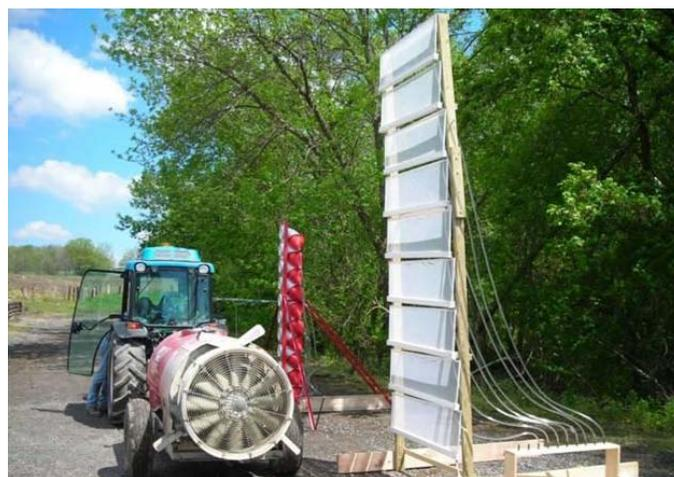
*Figure 6: Inexpensive patternator built out of window screens. Plans are available at:
