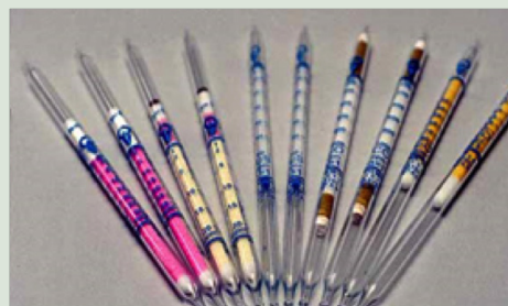
A wide variety of inexpensive gas detection tubes, used in the mining industry, are commercially available.
